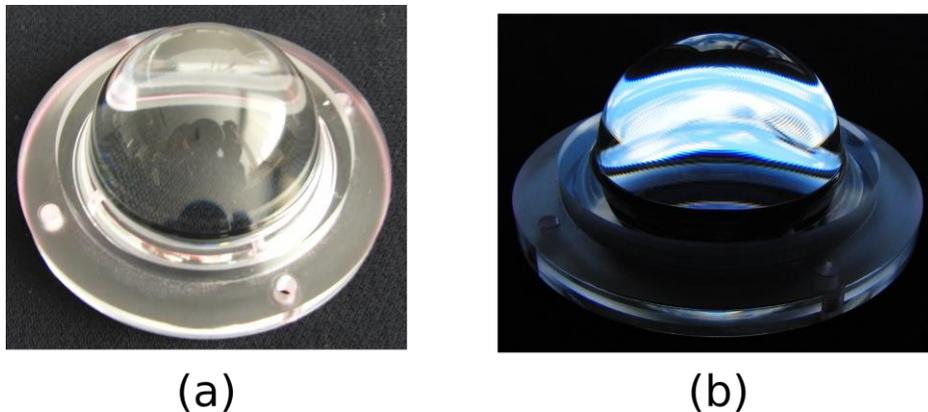
**Figure 2.** Photographs showing two views of the manufactured meniscus lens. The lens surface exhibits a low degree of scattering, but has periodic features that look much like a Fresnel lens imposed on the spherical surface shape, as is evident in subfigure (b). Surface profile measurements later confirmed that these errors are present only on the concave side of the lens, and are  $\sim 1\mu\text{m}$  in amplitude, with a period of about  $450\mu\text{m}$ .
