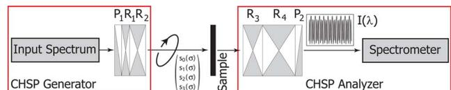
Fig. 1. (Color online) Basic layout of the snapshot Mueller matrix spectropolarimeter. Retarders 1 and 4 have their fast axes oriented at  $45^\circ$ , retarders 2 and 3 at  $0^\circ$ . Polarizers 1 and 2 both have their transmission axes oriented at  $0^\circ$ . CHSP, channeled spectropolarimeter.
